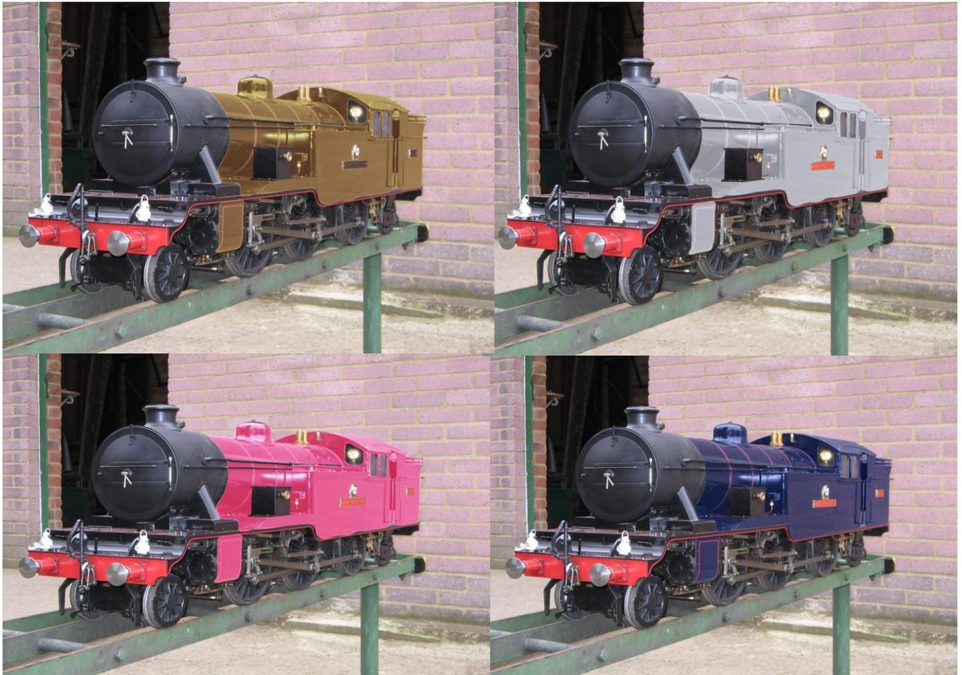
With colours decided upon, and the paint ordered, my workshop was converted into a spray shop for the duration of the task. When the paint arrived, all of the blue was sprayed, with several coats, and the black was sprayed from an aerosol can, again with several coats. The red lining was a Letraset lining tape, which must subsequently be varnished with a few coats of varnish.
