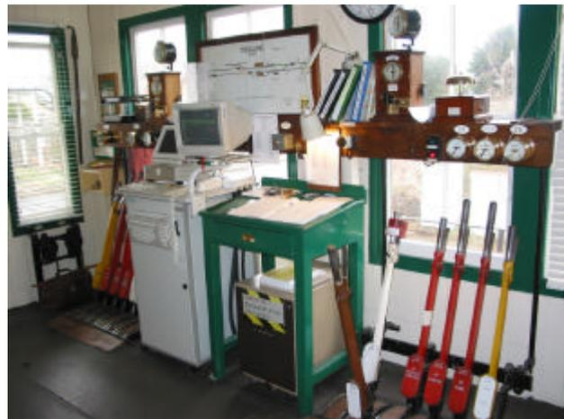
There was a time when the box would have been in charge of a number of goods sidings, and the missing levers would have operated the points and the signals associated with these sidings. The track diagram is much simpler now, and even though there is still a couple of trailing crossovers either end of the station, these are no longer controlled by the box.
