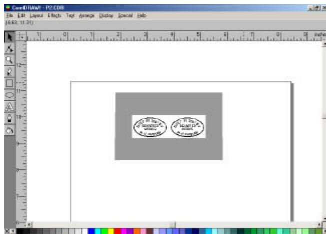
as this program allows text to be flowed to any shape and is ideal for laying out curved plates or oval works plates. With the thousands of text fonts available on a PC, it is easy to find one that is a match for the lettering required. Generally, I draw the plate at full size, although it can be drawn larger and scaled down to the required size at the printing stage.
