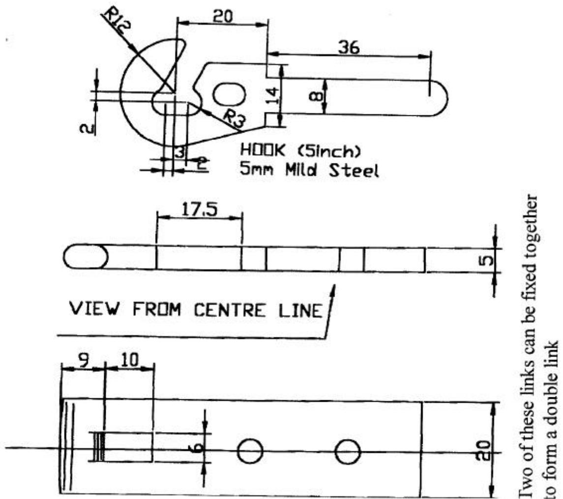
On my travels around various Model Railways, I have seen many steam, electric and other forms of engines. Some were connected to their carriages etc. by means of a chain, and others with a solid link. We all know that you cannot use a link on a normal hook, as when you stop, the link could, and possibly would, slide up out of the hook, thus causing a disaster as all the carriages you were pulling would try to climb all over you.
