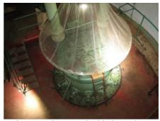
The gas exhauster shield above the main valve work
