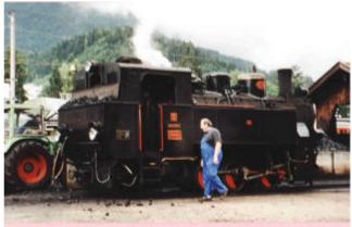
The other side of No.5. just after coaling up by the JCB type tractor just behind the engine. The Lenz poppet valve gear driven by the Walschearts' valve gear more clearly seen in this view.
