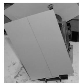
Line up the second card to the rail head inner surface and draw a line up to meet the centre line drawn previously.
