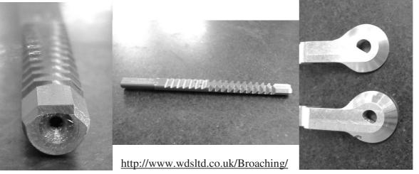
Pictures here show the Push-Broach (supplied by WDS MARLCO) and the lever before and after broaching.
