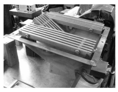
Four radiant super heaters have been constructed, and the boiler cladding is being assembled. Also the cab and running plates are in hand.
