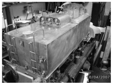
2007. Tender body: all brass soft soldered with baffle plates etc. This is almost complete, with working cupboards and coal hood to finish. This front section will also lift out to allow driving access.
